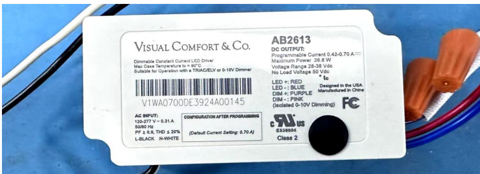
View of LED driver PSS30W-0700-38-VCC1 (AB2613)
